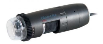
The Dino-Lite Edge models provide superior image quality and a high level of flexibility due to the adaptable cap design. The built-in adjustable polarizer reduces glare and reflection on shiny objects.
